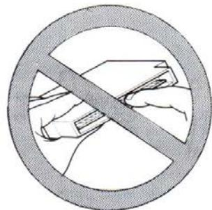
5. Before inserting a Game Pak, always check the Game Pak edge connector and remove any foreign materials. In order to keep the contacts clean, avoid touching the connector with your fingers.
