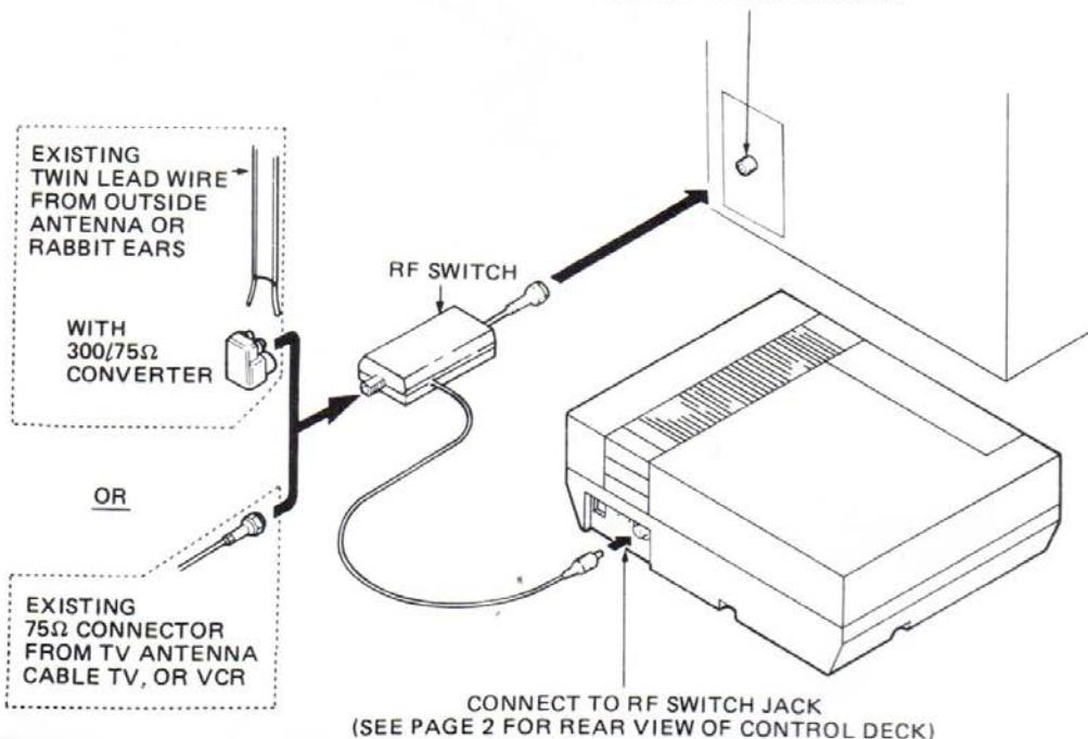
NOTE: If a VCR is already connected between the antenna and the VHF terminals on the back of your TV set, the RF Switch MUST be installed BETWEEN the VCR and the TV as shown below:
